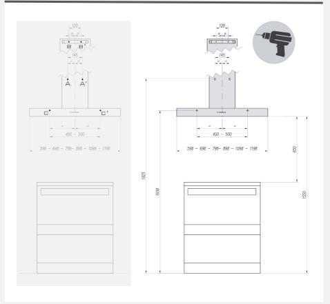
Hood must be fitted on minimum 5" Round ducting or rectangular equivalent
